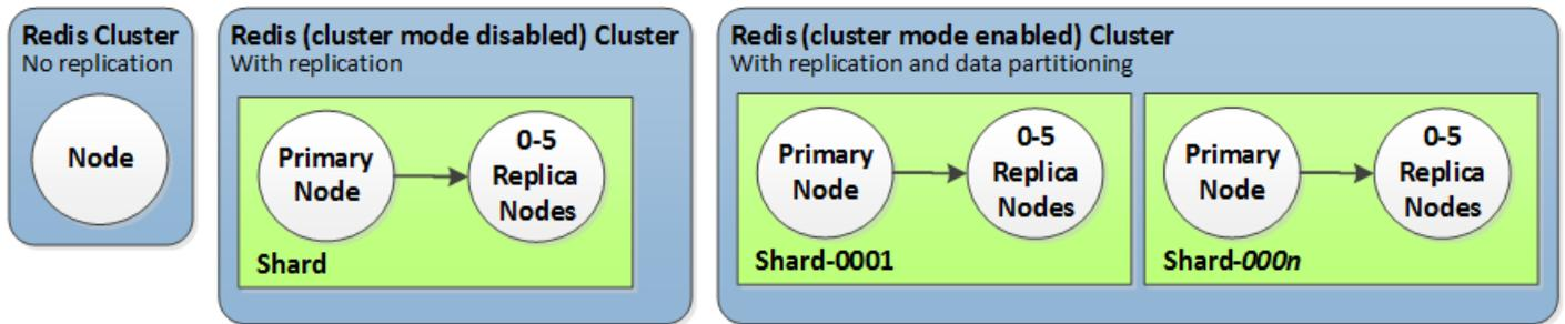
Most ElastiCache operations are performed at the cluster level. You can set up a cluster with a specific number of nodes and a parameter group that controls the properties for each node. All nodes within a cluster are designed to be of the same node type and have the same parameter and security group settings.
