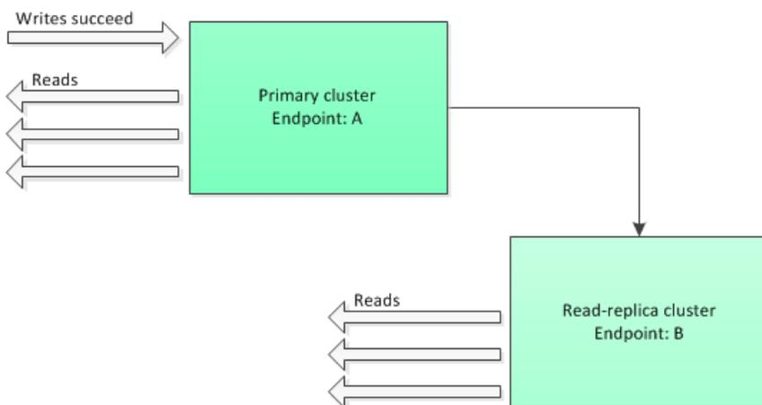
If the read-replica cluster is promoted to primary for any reason other than a Multi-AZ enabled replication group failing over, the client will continue trying to write to endpoint A. Because endpoint A is now the endpoint for a read-replica, these writes will fail. This is the behavior for Redis before ElastiCache introducing `close-on-replica-write` and the behavior if you disable `close-on-replica-write`.
