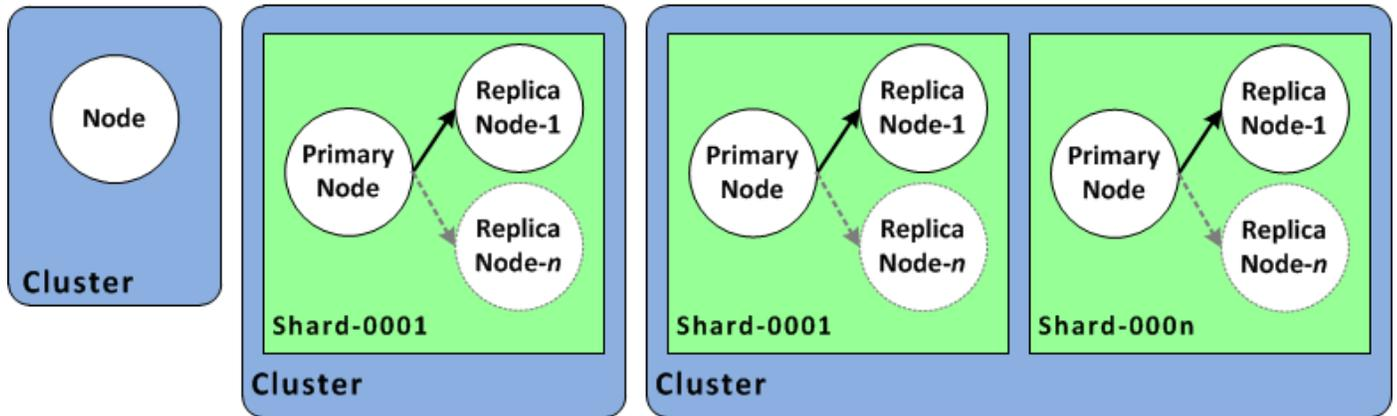
The ElastiCache API and AWS CLI operations still distinguish single node ElastiCache for Redis clusters from multi-node replication groups. The following diagram illustrates the various ElastiCache for Redis topologies from the ElastiCache API and AWS CLI perspective.
