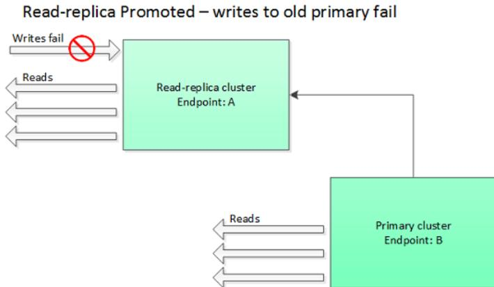
With `close-on-replica-write` enabled, any time a client attempts to write to a read-replica, the client connection to the cluster is closed. Your application logic should detect the disconnection, check the DNS table, and reconnect to the primary endpoint, which now would be endpoint B.
