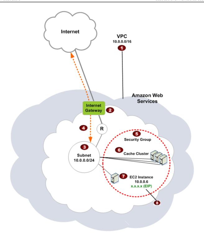
The Amazon VPC is an isolated portion of the AWS Cloud that is assigned its own block of IP addresses.
